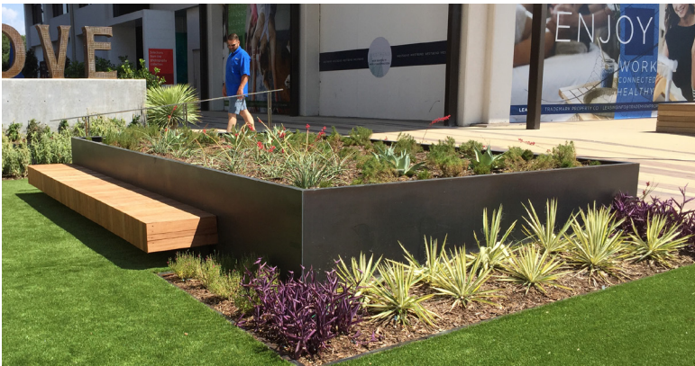
Typical Pre-Weathered Finish for Cor-Ten Steel
