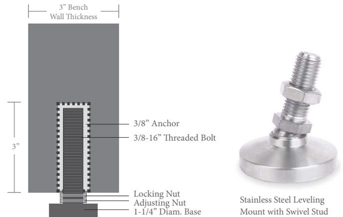
Stainless Steel Leveling Mount with Swivel Stud
