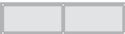
BX_BCH_8 96"L x 24"W x 18"H Intermediate Support (6) SS leveling feet per unit
